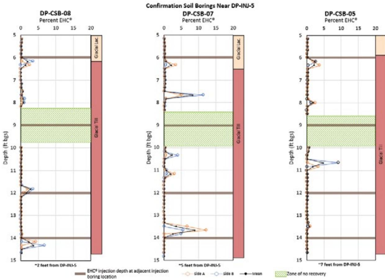
**Figure 3:** Example MS measurements in three soil cores. DP-CSB-08 was obtained adjacent to injection location DP-INJ-5. Actual injection intervals in DP-INJ-5 are also shown. DP-CSB-07 and DP-CSB-05 were obtained five and seven feet from the injection location, respectively.
