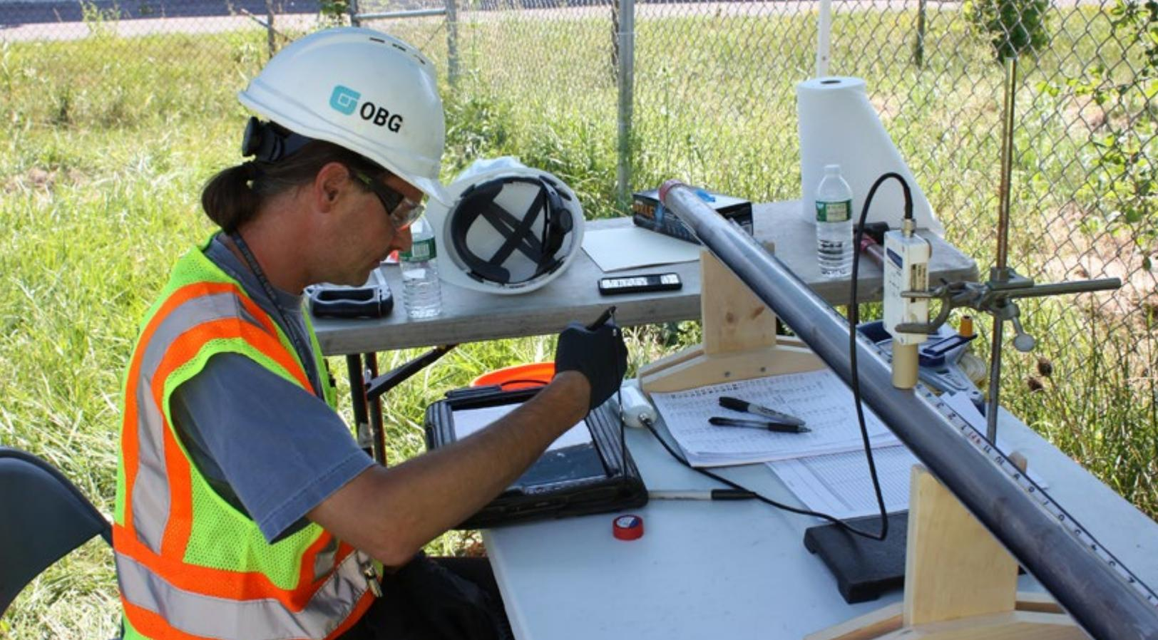
Figure 2: MS measurements being obtained on soil core.
