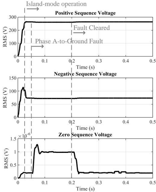
Fig. 8. Positive, negative, and zero sequences of voltage at PCC of PV plant 1.
