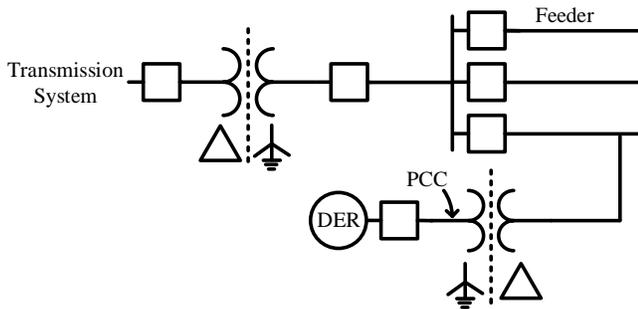
Fig. 1. Typical EDS with interconnected DER.
