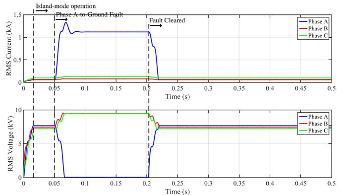
Fig. 6. Current and voltage at fault location.
