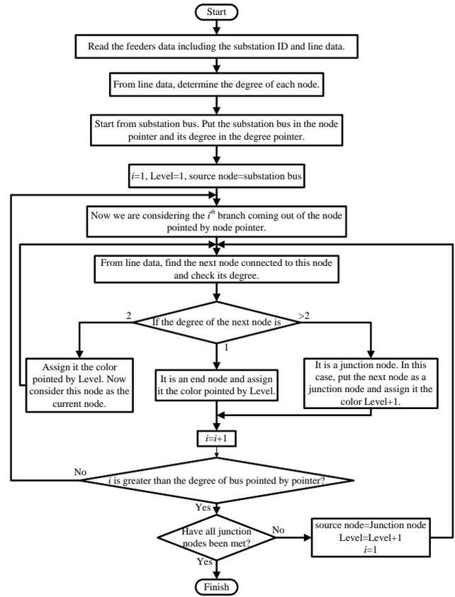
Fig. 3. Flowchart of assigning color to each node.
