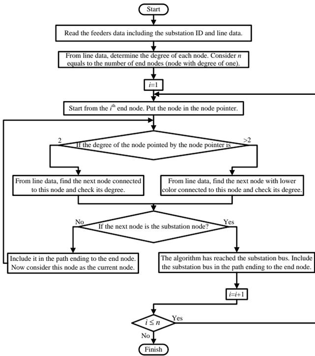
Fig. 4. Flowchart of tracking all paths from each end node to the source node.
