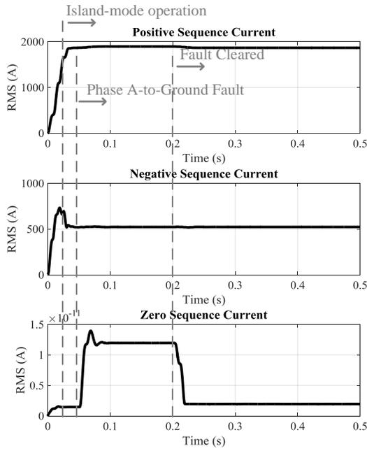
Fig. 7. Positive, negative, and zero sequences of current at PCC of PV plant 1.
