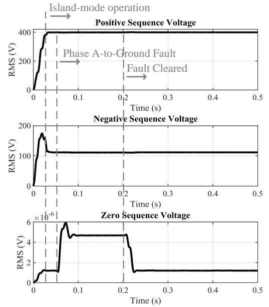
Fig. 9. Positive, negative, and zero sequences of voltage at PCC of PV plant 2.
