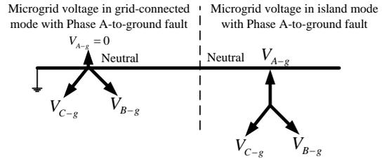
Fig. 2. Voltage level of a microgrid during a phase-to-ground fault.
