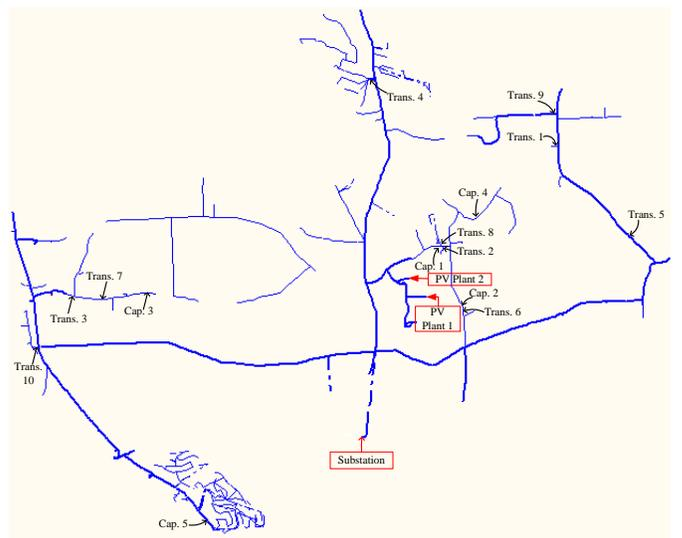
Fig. 5. Single line diagram of the distribution feeder.
