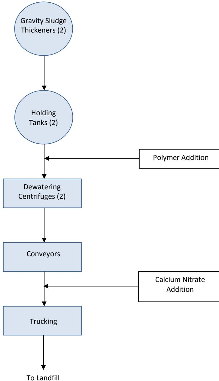
Figure 1: Northwest Quadrant WRRF Solids Handling
